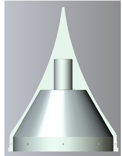
Fig 23: Modified hollow reflector design reduces thermal mass and lorentz forces
