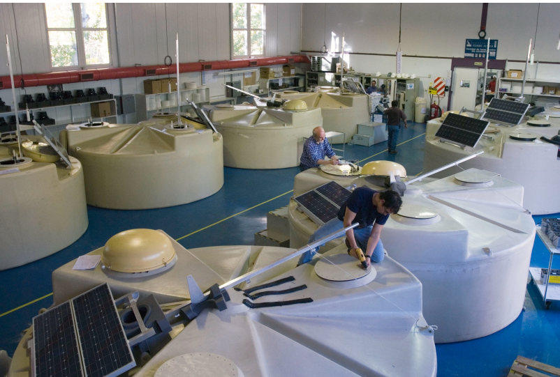
Assembling SD stations
