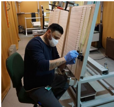
Assembling optical coupling
